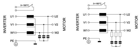
The temperature switch (normally closed) is mounted within the middle winding and opens at 180°C.
