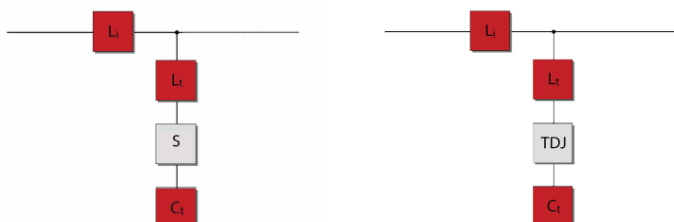
Figure 2 Filter configurations for FN3471, FN3473, FN3481 and FN3483
