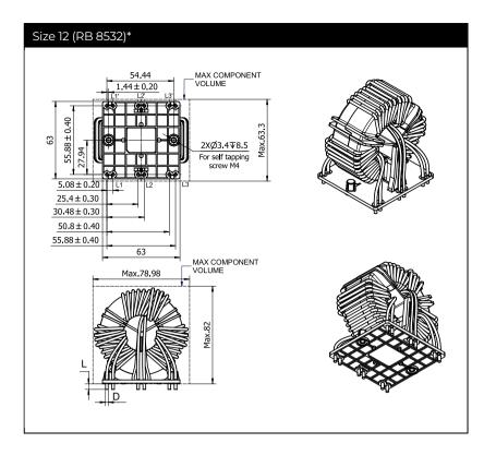
\* These choke sizes do have two parallel wires. Due to manufacturing processes and to cover current ampacity of chokes with high current rating, the number of parallel wires does vary between different sizes.
